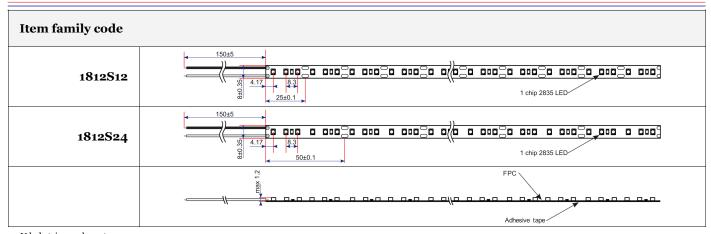
12V led strip can be cut every 25 mm 24V led strip can be cut every 50mm
